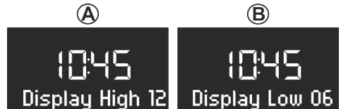
Fig. 16: Setting display dimmer
