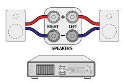
► Make sure that the speaker cables are correctly assigned to the connections on the unit. Note the orientation (right/left) and the polarity (+/-).
