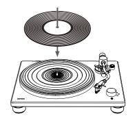
► To play 7-inch (17cm) records (EP records), place the supplied 45 RPM. adapter on the spindle.
